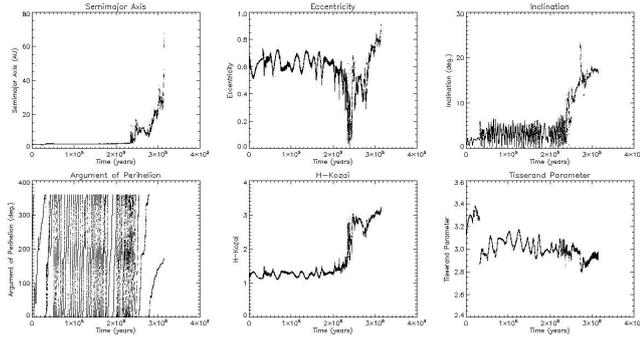
Figure 1. The evolution of the orbital elements of 4179 Toutatis asteroid over more than 300,000 years from  $t=0$ . The leaps in value of the semimajor axis are caused by close-encounter events with the major planets, from Venus to Uranus. In fact, a close-encounter will lead to a leap in value for all the orbital elements, not only for the semimajor axis but for the eccentricity and inclination as well (Siregar & Soegiartini, 2012).
