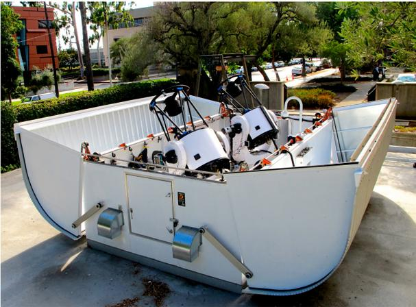
Figure 1. MINERVA commissioning site on the Caltech campus showing the open Aqawan and telescopes 1 and 2 inside.
