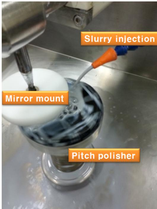
Figure 2. Pitch polisher, mirror mount and slurry injection system for polishing flat optical surfaces
