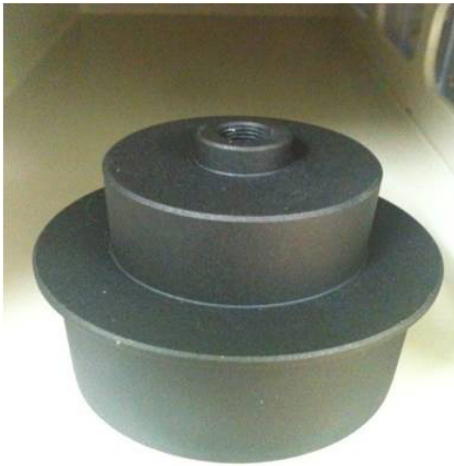
Figure 1. New adaptor to install spectrometer into telescope.
