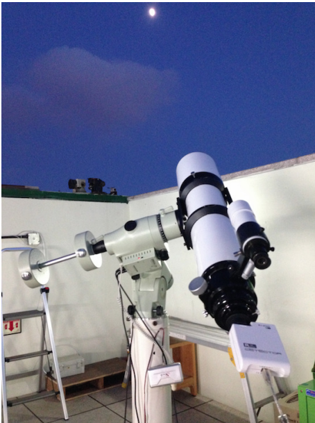
Figure 2. Installed spectrometer in a 5-inch refractor telescope.
